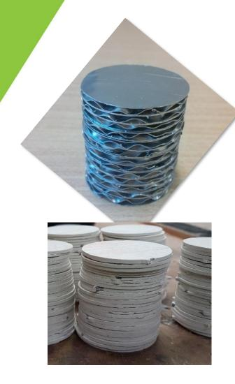
The sample format required for AS1530.1 testing is a cylinder, 45mm diameter and 50mm high. For thin sheets this is built up using several layers.
