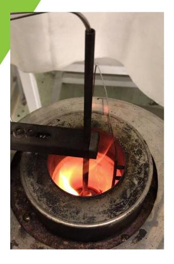
The solid FR core did not pass the AS1530.1 test. Due to significant flaming the testing was stopped. The FR core was deemed combustible to AS1530.1.
