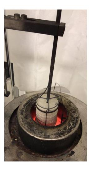
The AS1530.1 test procedure is to place into a furnace at 750C for 30 minutes.
